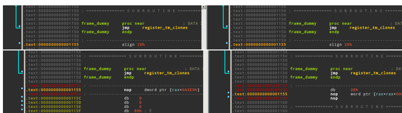
Fig. 2: Hiding the jump in a dummy application (backdoored version on the left)
